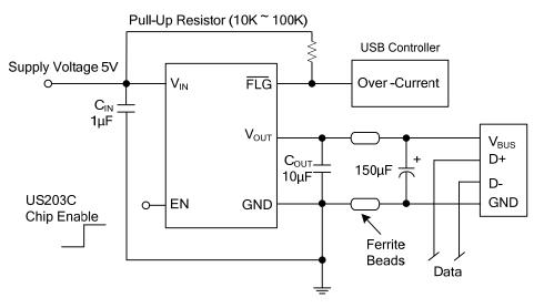
Note: A low-ESR 150 $\mu$ F aluminum electrolytic or tantalum between  $V_{\text{OUT}}$  and GND is strongly recommended to meet the 330mV maximum droop requirement in the hub  $V_{\text{BUS}}$ . (see Application Information Section for further details)
